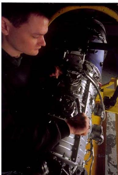
Getting the torque settings right on the hundreds of threaded fasteners involved in the rebuild of an aircraft engine is vital.
