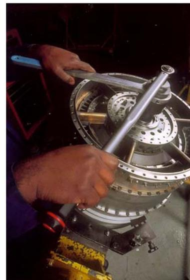
Engines typically overhauled by Sigma included the massive 22,100 lb thrust Rolls Royce Conway, the first bypass turbo fan engine put in to service by Rolls Royce, used on the mighty VC10 that started flying in the early 1960s. the T56/A15 turbo prop engines used on the ageless Hercules are also regular sights in Sigma's workshops, and some engines are still going strong 60 years after they were first built.
